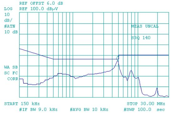
Fig. # 3 HT20 Filter with a Braided Ground
