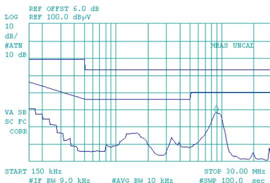
Fig. # 4 HT20 Input Filter & VHL25 Output Filter at Drive
