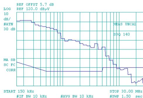
Fig. # 1 No filter 10 Amp load
